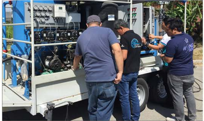
Laguna Water Technical Operations Team has undergone a training on how to operate the company's Mobile Treatment Plant (MTP). The MTP is designed to treat water sources and provide clean water during emergency situations.
